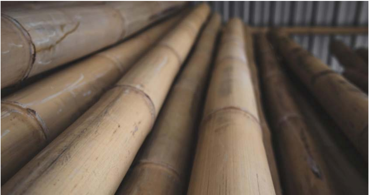
Bamboo petung poles of 6m length in preparation / drying at the warehouse.
