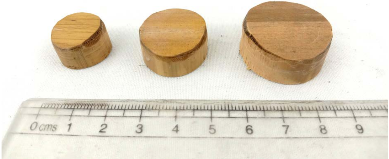
Cover bamboo for screws on top of the steel bars of 8, 10 and 12mm.
