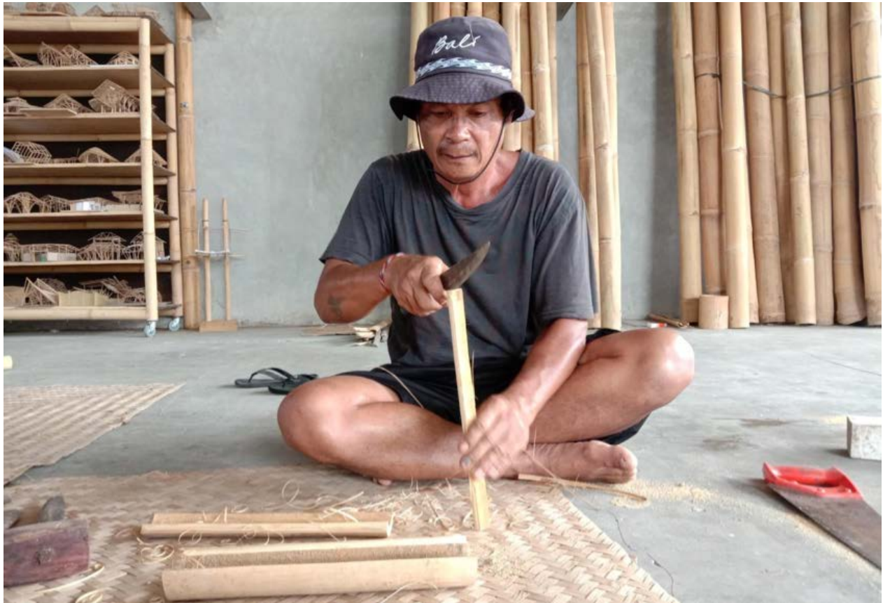
Bamboo pins fabrication process. Asali Bali. 2020.
