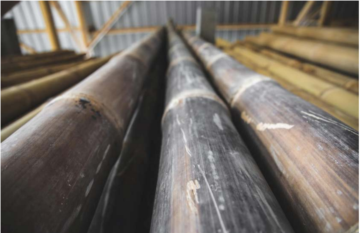
Black Petung for bamboo columns before finishing.
